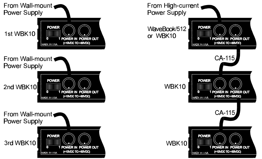
WBK10s with separate power supplies or WBK10s with daisy-chain power supplies WBK10 Cable Connections
